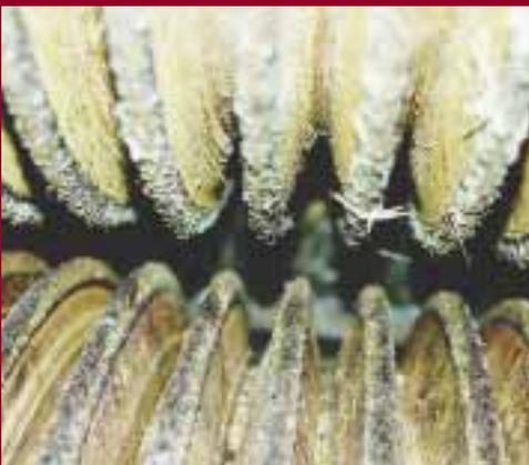
**#07:** The Top and Delivery rolls at Tully No. 2 mill in 1998. Having completed 1,000,000 tonnes to this point, with no maintenance.
