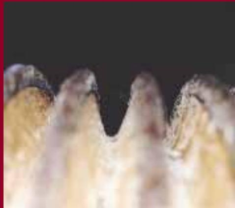
**#06:** The top roll at Tully in 1998 after 1.0 million tonnes. Note that the bottom of the grooves are not worn.
