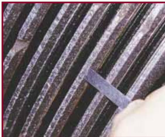
LEFT: The typical mill roll tooth profile used at South Johnstone Mill on the 1" pitch rolls. It was clearly not suitable to be used with the now patented A.R.M.\* Hardfacing process.
