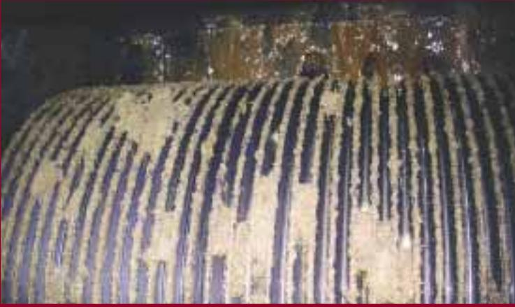
**#03:** The A.R.M.\* roll at Tully Mill in 1998, top roll No.2 Mill, after it had completed 1,000,000 tonnes – with no maintenance.
