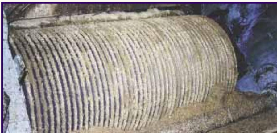
*#16: The A.R.M.\* Hardfaced top roll at Rocky Point Mill after 400,000 tonnes crushed, in the 2001 trials.*
