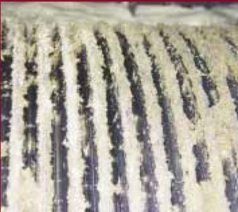
**#05:** The A.R.M.\* Hardfaced top roll No.4 Mill, Tully 1999-2000. Pictured here at 1.6 million tonnes with no maintenance. It went on to complete both the 1999 and 2000 seasons for a total of 3.2 million tonnes.
