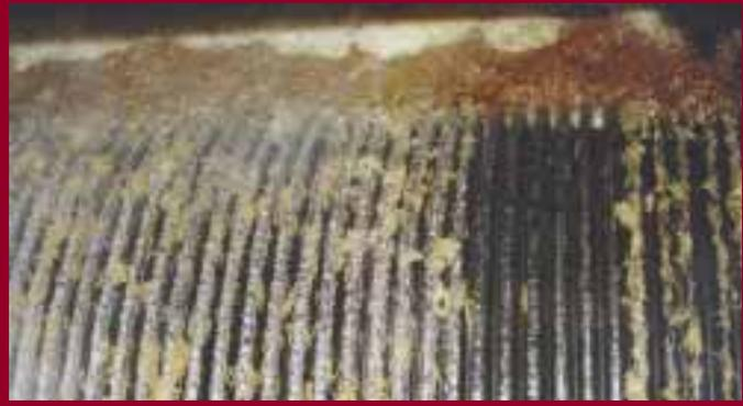
**#02:** South Johnstone Mill in 1997. Top roll No. 4 Mill. This is the standard chromium carbide hardfacing section (not the A.R.M.\* invention) which was re-hardfaced approximately 14 times during the trial, and lost about 25mm in diameter.
