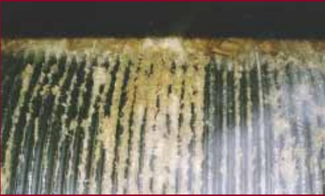
**#01:** Bagasse covered section of teeth after 1.0 million tonnes during 1997 at South Johnstone Mill with no maintenance (also see photo #14).
