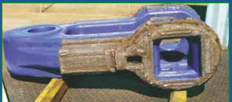
CQMS Drag Shackle, A.R.M.* Hardfaced to extend the operating life.
