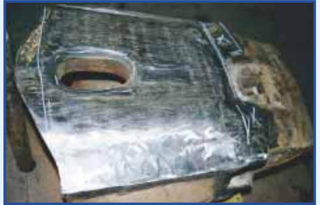
BEFORE: 130 series Dragline adapter prior to an A.R.M* rebuild.
