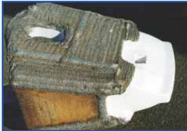
AFTER: The same adapter after an A.R.M* rebuild which cost less than 30% of a new adapter price for a complete second life cycle.
