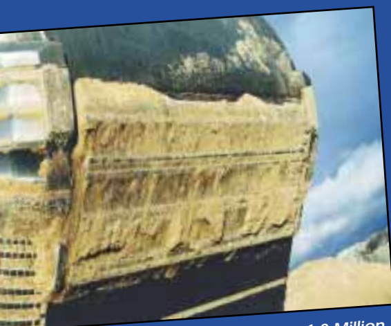
* Dragline Bucket Heel Package after 1.0 Million (Previously 40mm Bis 80 only lasted 1.3 Million before holes appeared in the floor).
